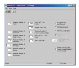
CMX-RTX and CMX-Tiny+ are truly preemptive, multi-tasking real time operating systems (RTOS) for the Atmel series of processors. These "lean and mean" RTOSes offer the smallest footprint, the fastest context switching times, and the lowest interrupt latency times available on the market today. While CMX-RTX and CMX-Tiny+ are a fully preemptive RTOS, support is also provided for cooperative scheduling or time-slicing, if desired.
